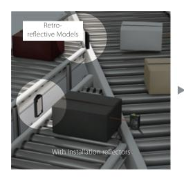
Although retro-reflective sensors are used for long-distance sensing in converging and diverging lines, space may be in a issue for mounting reflectors.
