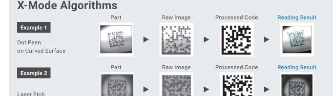
X-Mode algorithms ensures that all Direct "Part Marks can be read as easily as a printed label.
