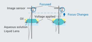
Predictive autofocus automatically adjust for the distance the barcode reader is from the surface and makes reading various sizes of codes, simple. The V460's incredible ability to automatically read a broad range of challenging direct part marks and printed labels without adjustment, is built upon three key technologies: predictive autofocus, X-Mode decoding algorithms, and intelligent lighting.
